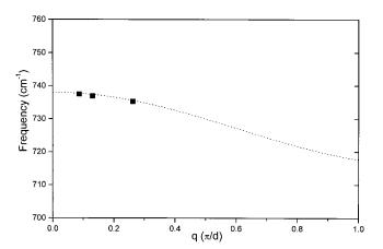
FIG. 3. The measured  $A_1$ (LO) phonon frequency in GaN/Al<sub>0.2</sub>Ga<sub>0.8</sub>N superlattices. The dot line is the calculated curve from Ref. 22.
