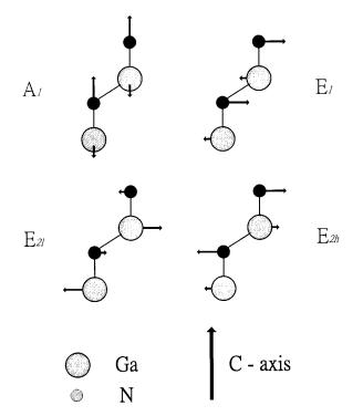
FIG. 2. Raman active optical modes in the wurtzite structure,  $E_{2i}$  and  $E_{2b}$  correspond to the low- and high-frequency  $E_2$  modes, respectively.
