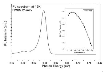
FIG. 4. The photoluminescence from the superlattice with well width 36 Å at 15 K. The peak at 3.565 eV is due to the emission from the GaN wells. The inset shows the temperature dependence of PL peak position of the GaN/Al<sub>0.2</sub>Ga<sub>0.8</sub>N superlattices.
