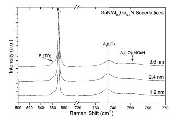
FIG. 1. Room-temperature Raman spectra of GaN/Al\_{0.2}Ga\_{0.8}N superlattices with different well widths given in the figure.
